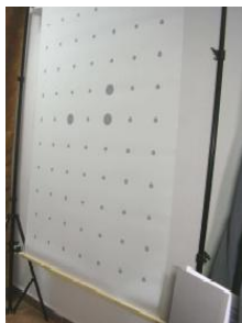
Fig. 4: Panel with holes placed at calibrated distances
