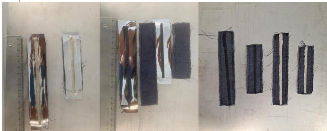
Fig. 2: Screen printing of the textile substrate with the two types of paste
