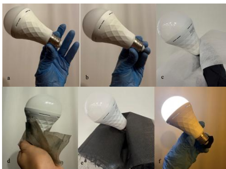
Fig.4. The digital photographs showing the gloves (a, b), NW (c), D-GO-NW (d), and B-GO-NW (e) do not light the LED, while the ROP-RGO-NW-2 sample lights the LED.
