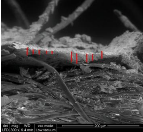
Fig. 3: Measured thickness of the 100 mm Ag coating
